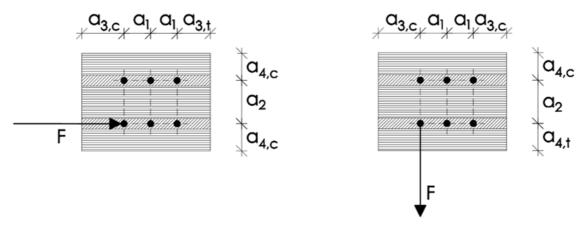
For screws in the edge surface,  $a_1$  and  $a_3$  are parallel to the CLT plane surface,  $a_2$  and  $a_4$  perpendicular to CLT plane surface.
