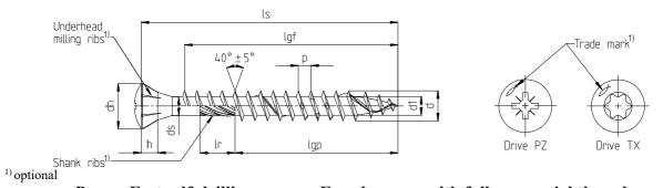
Power-Fast self-drilling screw - Facade screw with full- or partial thread
