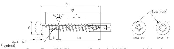
Power-Fast self-drilling screw - Pan head with full- or partial thread
