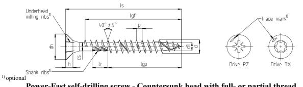
Power-Fast self-drilling screw - Countersunk head with full- or partial thread
