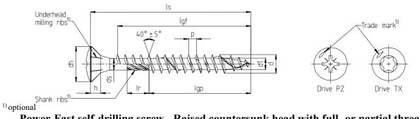
Power-Fast self-drilling screw - Raised countersunk head with full- or partial thread
