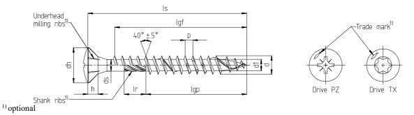
Power-Fast self-drilling screw - Raised countersunk head with full- or partial thread
