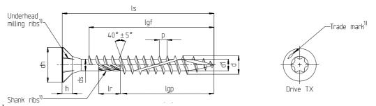
FCS wood construction screw - Countersunk head with full- or partial thread
