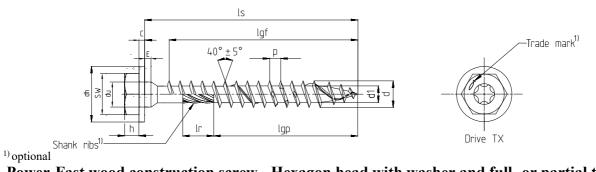
Power-Fast wood construction screw - Hexagon head with washer and full- or partial thread
