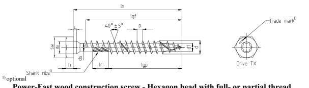
Power-Fast wood construction screw - Hexagon head with full- or partial thread
