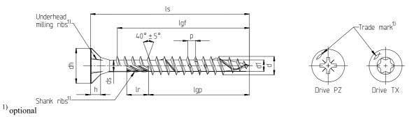
Power-Fast wood construction screw - Countersunk head with full- or partial thread
